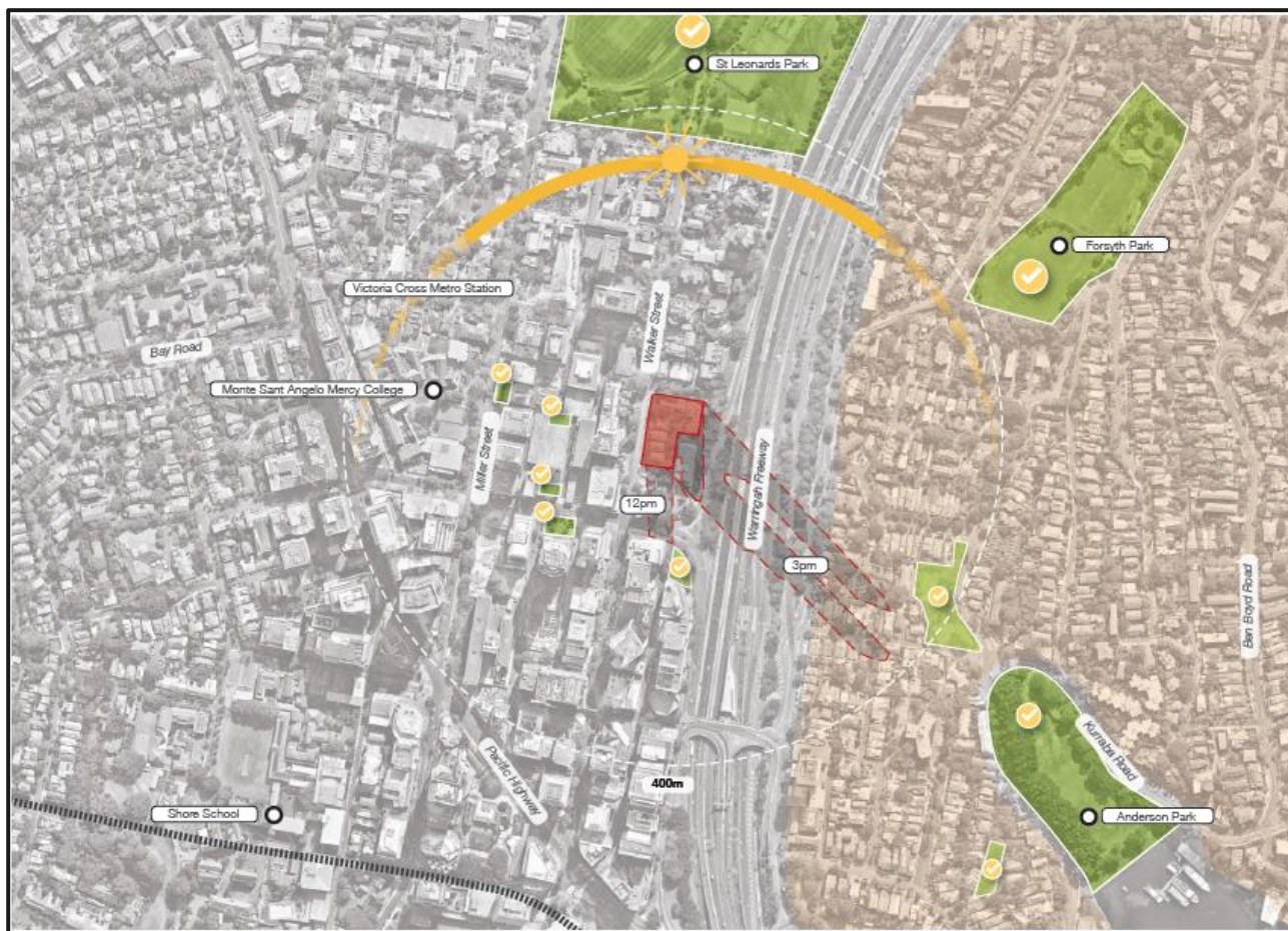
Figure 35: Solar access study showing the priority zones
